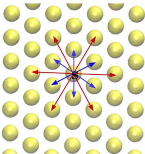
**Figure S2.** The hexagonal arrangement of Sulfur atoms (yellow) on the Au layer (omitted for clarity). For each S atom, the next nearest neighbour (NNN, red arrow) S atoms are at  $\pm 0^\circ$ ,  $\pm 60^\circ$ ,  $\pm 120^\circ$ ,  $\pm 180^\circ$  directions; the nearest neighbour (NN, blue arrow) S atoms are at  $\pm 30^\circ$ ,  $\pm 90^\circ$  and  $\pm 150^\circ$  directions.
