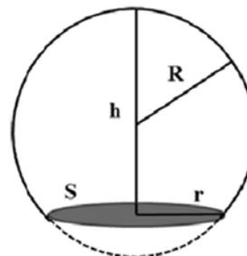
Figure S3. A geometric method to estimate droplet contact angle.
