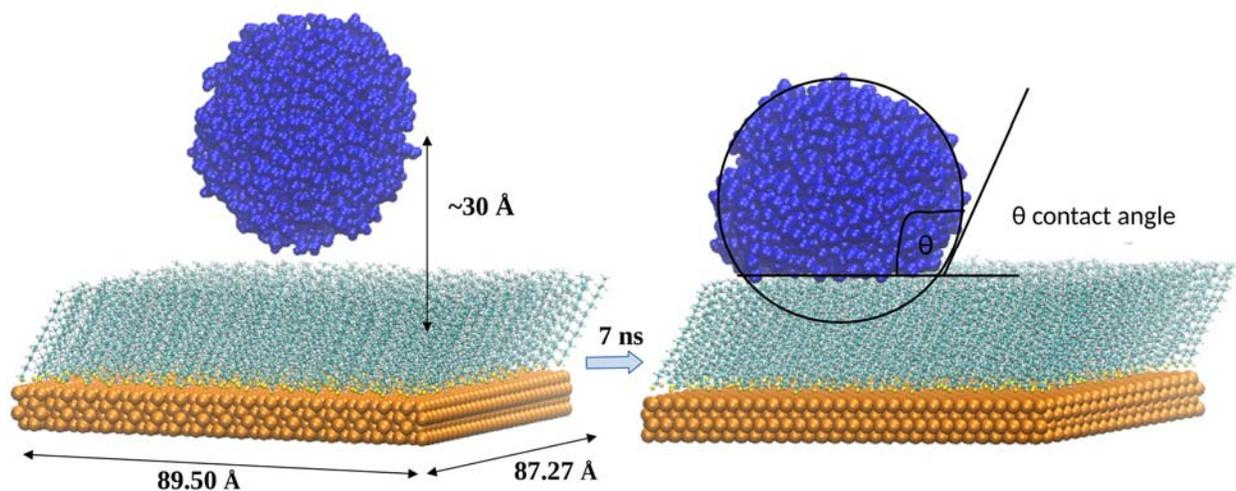
**Figure S1.** Snapshots of a droplet-SAM system with 1-Octadecanethiol ligands: Initial structure (left) and equilibrated structure after 7 ns of simulation time (right). The water droplet sat on the monolayer surface and stabilized with a contact angle ( $\theta$ ).
