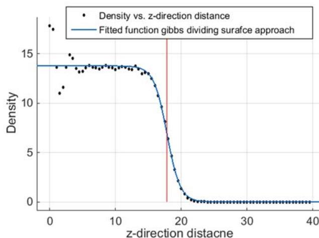
**Figure S4.** The hyperbolic tangent function (blue solid line) fitted to the water density profile (black dots). The  $Z$  location at the middle of the water-vapor interface is taken to be the height of the droplet.
